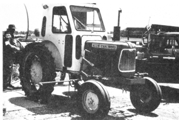
Figure 3. Closed-cab tractor utilized by applicator no. 3. In this case air samples were collected inside the cab.
