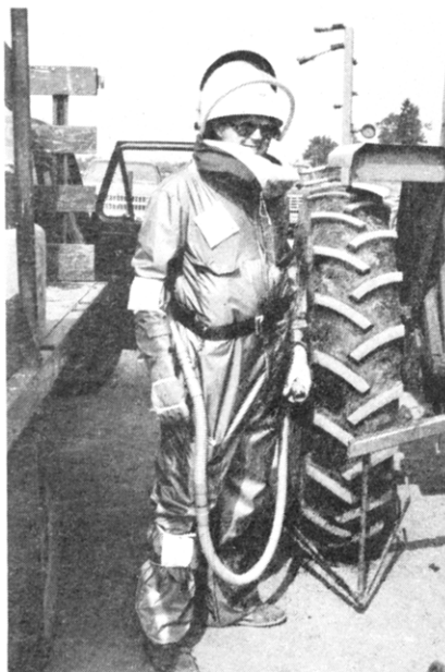
Figure 1. Applicator with Gore-Tex coverall especially designed and constructed for this study. Note location of gauze sampling pads on leg, arm, chest, and inside palm.
